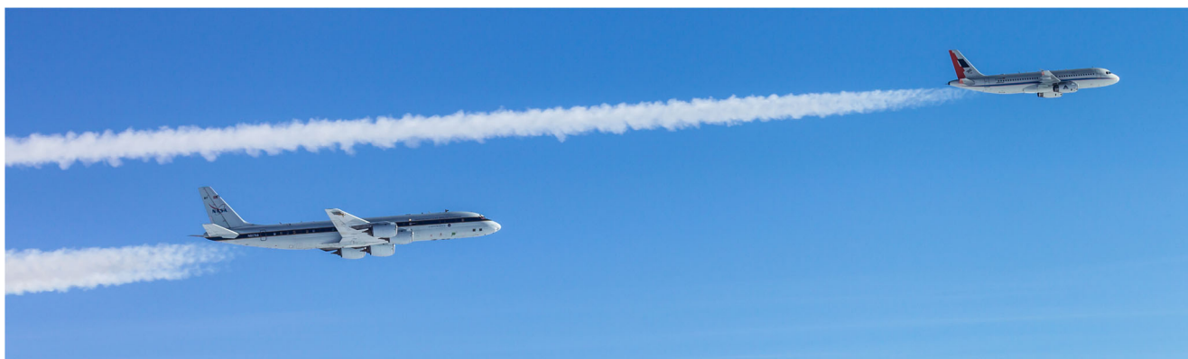
Fig. 1 The NASA DC8 research aircraft probing contrails from the DLR A320 burning sustainable aviation fuel blends. Photo showing the DC8 chasing a contrail from the A320 burning a sustainable aviation fuel blend above Germany on 24 January 2018.
